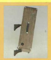
WALL MOUNTING BRACKETS can be left in place, speaker simply hooked on when needed. Lower assembly has slot and set screw for adjusting vertical angle. Brackets permit horizontal rotation.
