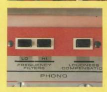
HI AND LOW FREQUENCY FILTERS in phono circuit reduce hiss and rumble from less-than-perfect records.
